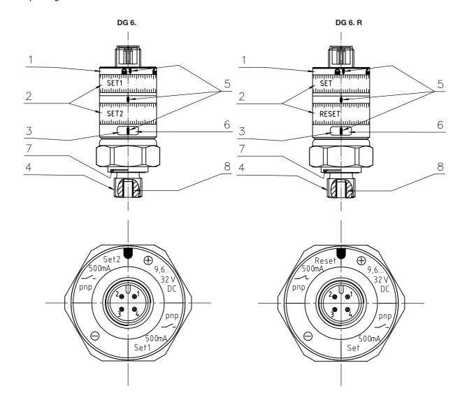
SET1 = Signal output NO-contact PIN 4 SET2 = Signal output NO-contact PIN 2
